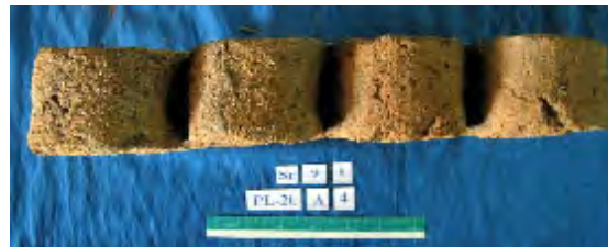
Fig. 61a and b: Top and plan view of unique “B”-shaped brick style used to create complex moldings on the profile.
